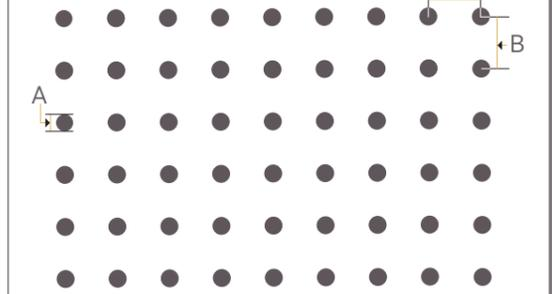
Even Pattern. Hole Size Dia (A): 1.5mm, Pitch (B): 4mm, Open Area: 11%
