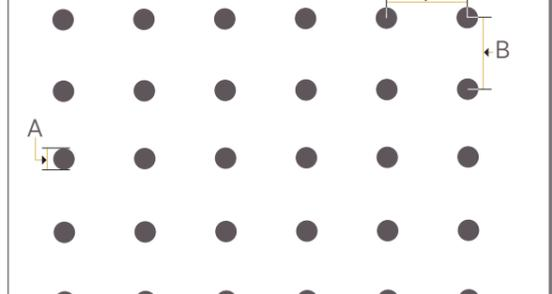
Even Pattern. Hole Size Dia (A): 2.5mm, Pitch (B): 5.5mm, Open Area: 16%
