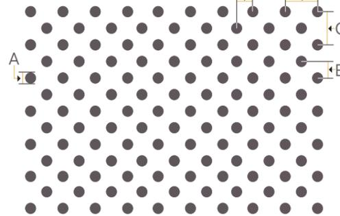
Diagonal Pattern. Hole Size Dia (A): 1.5mm, Pitch (B): 2mm, Pitch (C): 4mm, Open Area: 22%
