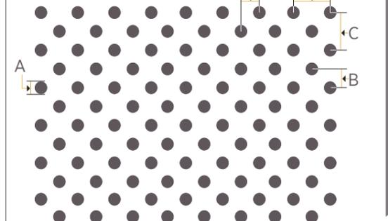
Diagonal Pattern. Hole Size Dia (A): 1.8mm, Pitch (B): 2.5mm, Pitch (C): 5mm, Open Area: 20%
