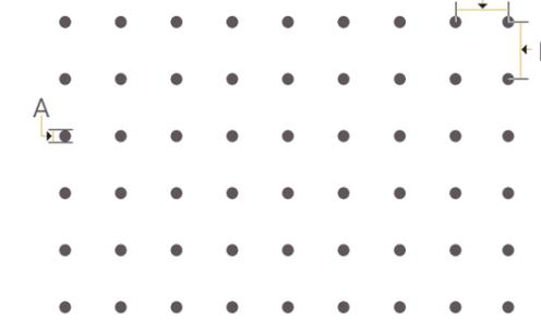
Even Pattern. Hole Size Dia (A): 0.75mm, Pitch (B): 5mm, Open Area: 1%
