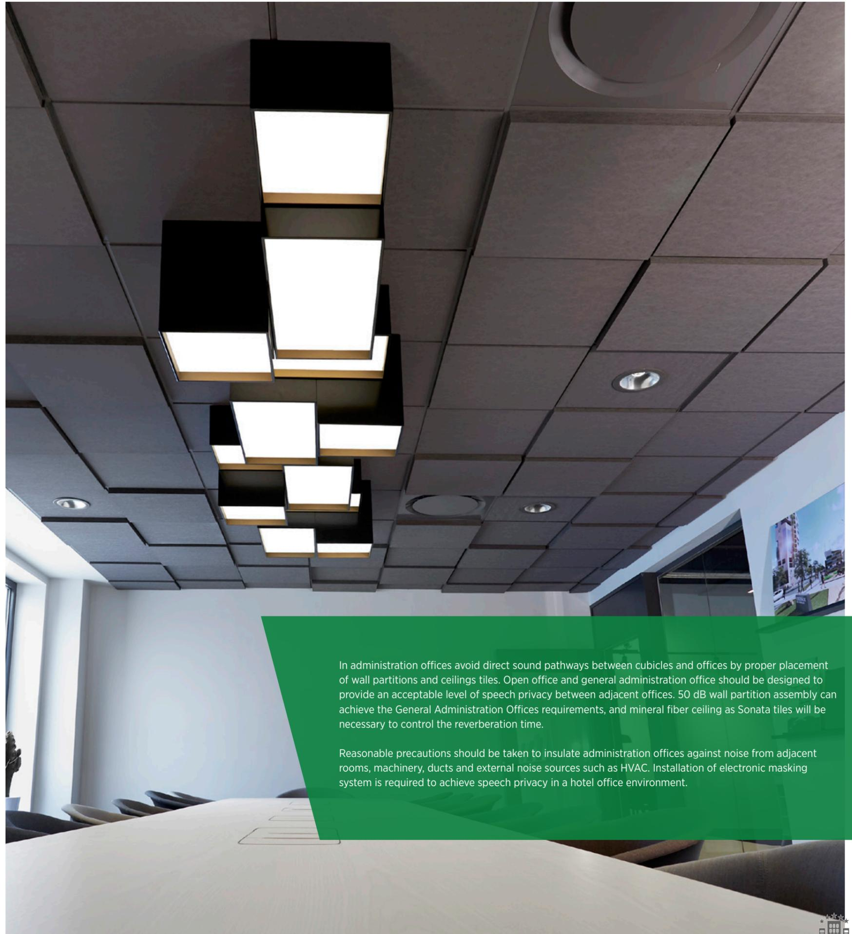
In administration offices avoid direct sound pathways between cubicles and offices by proper placement of wall partitions and ceiling tiles. Open office and general administration office should be designed to provide an acceptable level of speech privacy between adjacent offices. 50 dB wall partition assembly can achieve the General Administration Offices requirements, and mineral fiber ceiling as Sonata tiles will be necessary to control the reverberation time.
